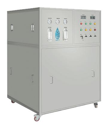
This machine has a small footprint, it can produce up to 250 liters of deionized water per hour. It has 3 main parts which are: Treatment, Reverse Osmosis, Resin bed.
