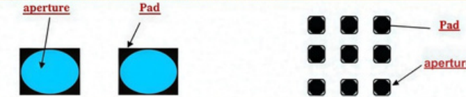
Figure: Opening Methods for 0402 Components & BGA
